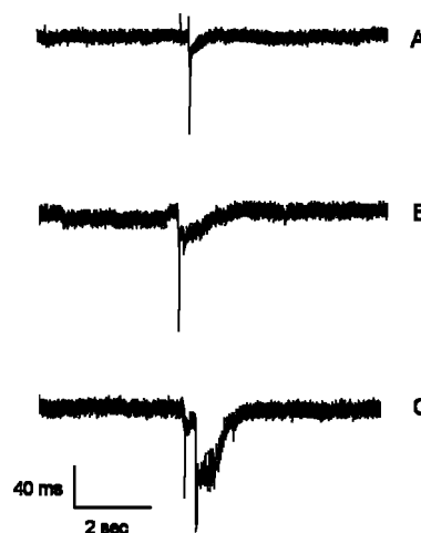
Figure 3. Expanded views of typical current pulses associated with tip-to-base translocation of (A) BSA, (B) PhB, and (C) \beta Gal, 100 nm protein. Tip diameter = 17 nm. Transmembrane potential = 1000 mV.
